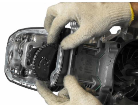
After removing the head the camshaft control components can be removed:
